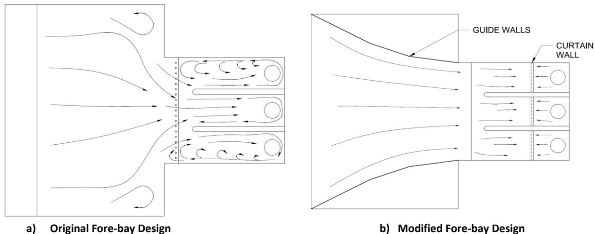
Figure 5 Modifications Involving Flow Guidance within Fore-bay
