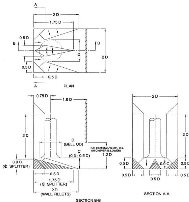
Figure 3 Common Fillet and Splitter Remedies
