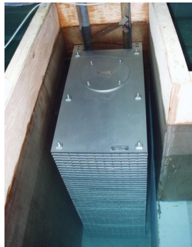
Figure 1 Typical stack of strainer disks. The circular section in the top covers the core tube.
