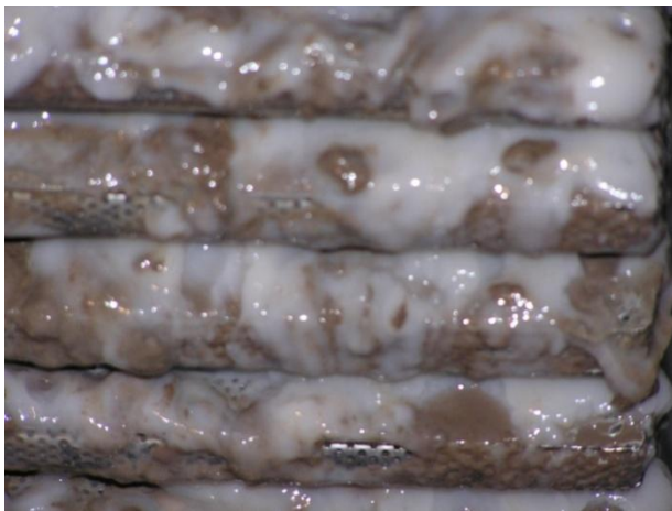
Figure 9 Side view of a strainer after head loss testing.
