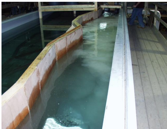
Figure 5 Temporary flume side walls adjusted to reproduce averaged approach flow velocities and gradients.
