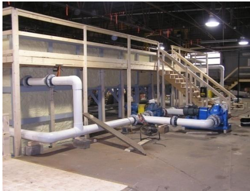
Figure 3 Photo of test flume and flow loop. View angle is similar to Figure 1, but from a lower elevation.
