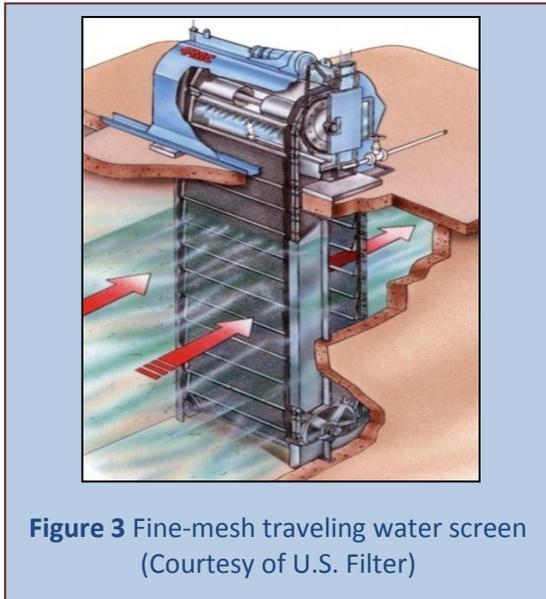
**Figure 3** Fine-mesh traveling water screen
