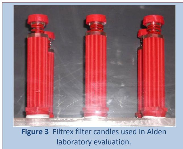
**Figure 3** Filtrex filter candles used in Alden laboratory evaluation.
