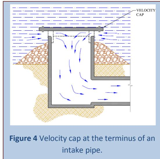
**Figure 4** Velocity cap at the terminus of an intake pipe.
