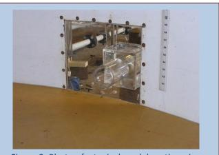
Figure 2. Photo of a typical model suction pipe
