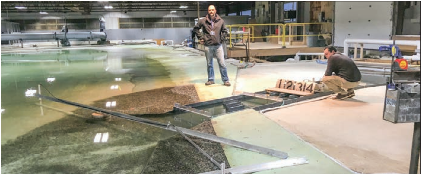
Brad Barth, standing, the Coastal Protection & Restoration Authority's operations assist administrator for the proposed Mid-Barataria Sediment Diversion, and an employee of Alden Labs, crouching, observe a 1:65 scale model of the diversion that takes up most of a 300-foot by 90-foot building in Holden, Mass. Alden built two huge models, one of the Mississippi River and one of the outfall in Barataria Bay, to study how the diversion will perform.
